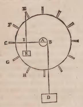
Suppose A B, for the Semidiameter of the Axis or Cylinder, and AC, for the Semidiameter of the rundle, with the spokes; then the power
